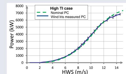
To investigate the effects of TI on the Power Curve (PC), high TI ( $TI > 12\%$ ) and low TI ( $TI < 12\%$ ) categories were created. For low TI, the measured PC was slightly above the nominal PC at high wind speed. However, for high TI, although the PC is slightly above the nominal PC from 6 to 11m/s, the turbine is underperforming at high wind speeds.
