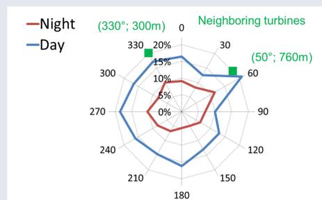
As could be expected from thermal effects during the spring season, TI is on average higher during the day (13.4%) than the night (8.6%). A day/night TI rose was built to analyze this for each sectors. It allows to visualize a wake effect for a similar size turbine located 760m away but not for a smaller one closer, at 300m.
