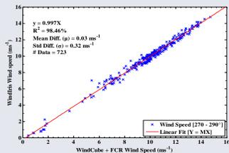
During this campaign, the Wind Iris was also validated against a WINDCUBE v2 installed 2.3D (290m) away from the turbine. The validation showed good results with slope near to 1 and  $R^2$  close to 0.99 (to be presented in a later publication).
