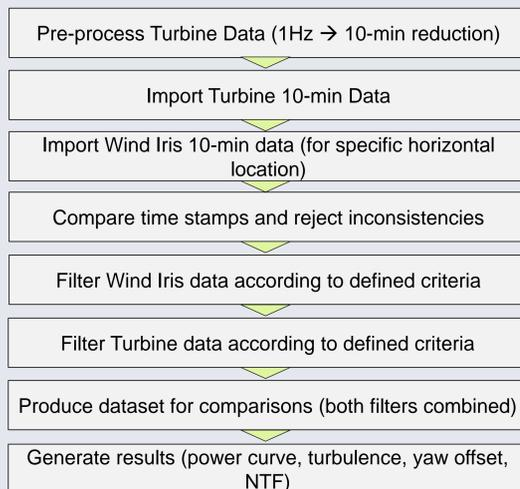
In order to support the analysis of the data derived from multiple measurement sources, a procedure was developed for automated data preprocessing. The result provided a high quality, properly synchronized dataset for further analysis.
