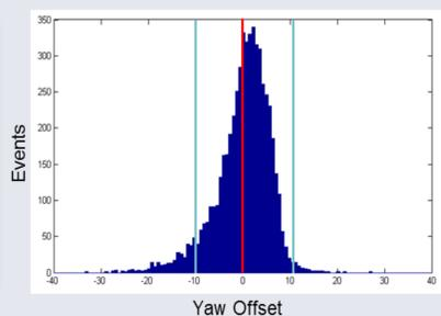
Within a few days, it was identified that the turbine did not suffer from significant yaw misalignment. The yaw offset distribution was found to be skewed, which in the present case is reflected by a higher number of large negative offsets than large positive offsets were observed.
