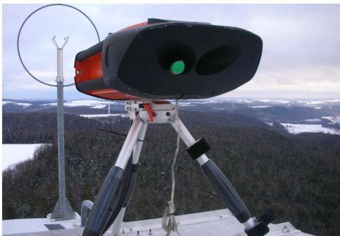
“We used the Wind Iris to determine whether there was yaw misalignment of one of our utility-scale wind turbines. By detecting and accurately quantifying the yaw misalignment, we were able to correct the error and gain significant AEP improvement. Based on this evaluation, First Wind decided to purchase a Wind Iris so we can optimize more turbines in our fleet”.
